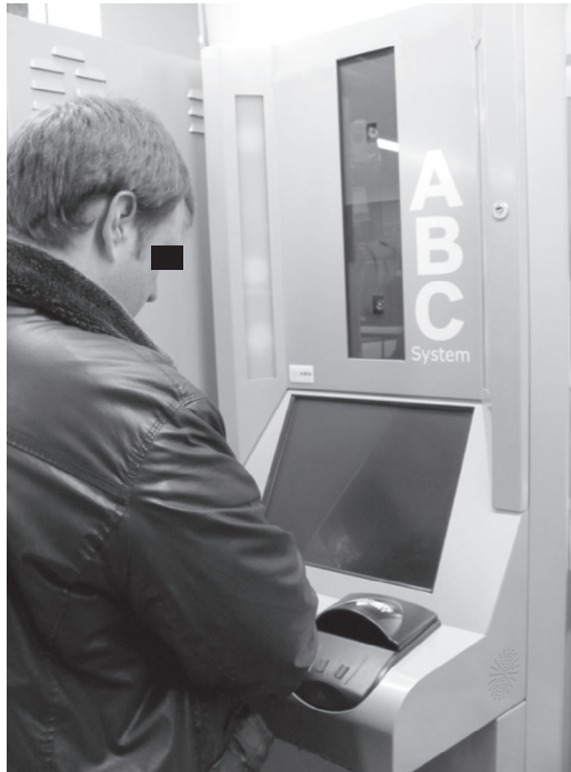
Fig. 7 – Experimental evaluation setup. The circles in front of the subject are the cameras that capture the face images, and those to the side (left and right) are the light emitters. Explanatory video screens, the fingerprint reader, and the e-MRTD are below the cameras.
